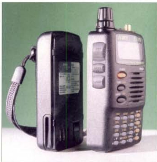
Fig. 1: The DJ-V5 comes complete with battery pack and here you can see it detached from the front of the radio.
