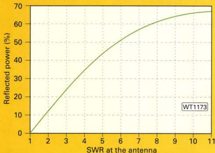
Fig. 1: This graph shows how the reflected power in the feeder rises with increase in the s.w.r. at the antenna/feeder interface.
