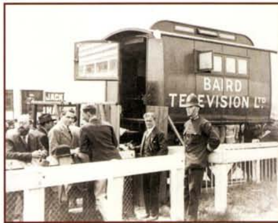
Fig. 3: The outside broadcast caravan at the 1931 Derby. Note: the hinged mirror on the door, which directed different scenes on to the TV equipment.
