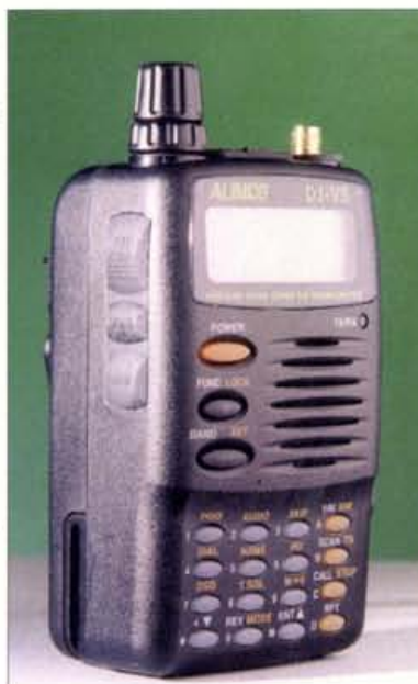
Fig. 3: Side view of the DJ-V5 which shows you the Press To Talk (PTT), Monitor (squelch defeat) and Lamp control buttons.
