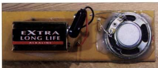
Fig. 4: Photograph showing simple method of attaching battery and small loudspeaker (1.5in, 38mm diameter) to the rear of the p.c.b. using rapid setting epoxy resin adhesive. Take care that the adhesive does not 'run' under the speaker rim onto the paper cone, but only onto the metal rim of the speaker frame.
