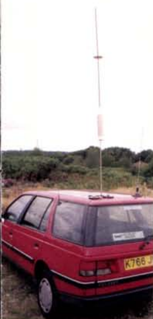
Fig. 2: Rear 'side on' view of G3XFD's car to illustrate the size of the 'Bugcatcher'.
