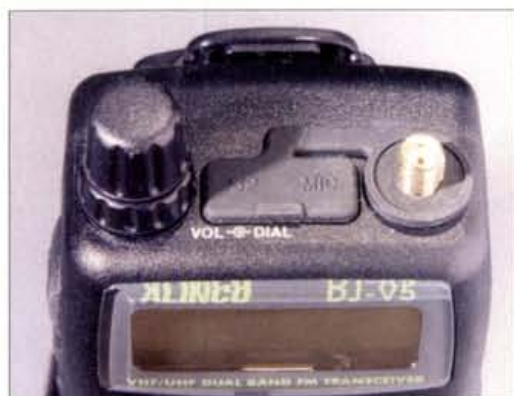
Fig. 2: Top view of the Alinco. "... the antenna connection is an SMA type and the radio has the familiar 3.5/2.5mm jack socket-pair for the speaker/microphone extension on the top of the transceiver".
