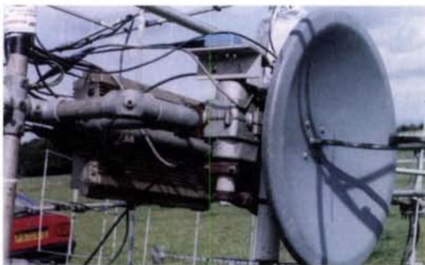
Fig. 1: "Serious hardware" department. A 10GHz microwave dish ready for an ATV contest as part of the Severnside ATV Group's antenna array.
