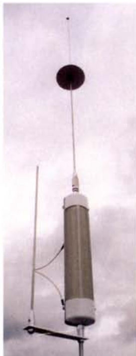
The 'Texas Bugcatcher' h.f. mobile antenna, with large diameter loading coil, capacity 'hat' and the vertical 50MHz 'add-on' element.
