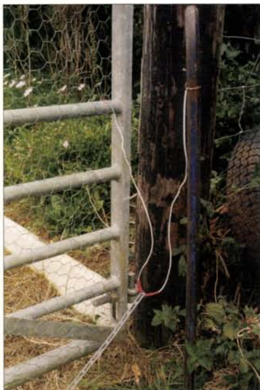
A metal gate set on a wooden post could be a suitable hidden antenna. Note: the wiring joints are for illustration purposes only and should be far more secure in a permanent installation. (For use in your own property only - for safety reasons).
